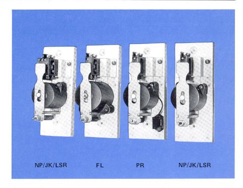
The contacts are bridge-type, double-breaking, silver cadmium oxide consisting of one (1) normally open (N.O.) and one (1) normally closed (N.C.) set of contacts in a common assembly block.
