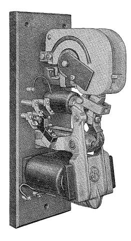
OPERATING COILS: These contactors will operate satisfactorily on 80% of normal control voltage when the coils are hot and will hold in on 20% of normal voltage. The coils will stand 110% of normal voltage continuously.
