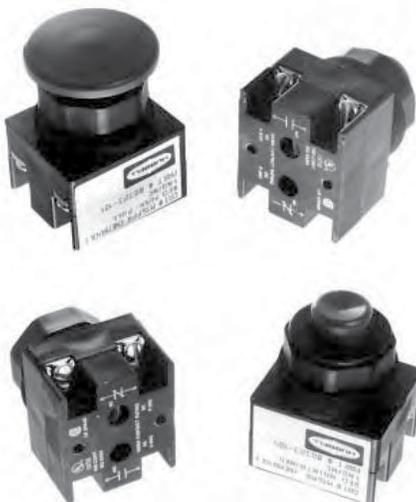
Hubbell's maintained pushbuttons are available in two variations. Single button mushroom head "push/pull" units are stand alone buttons that are commonly used for a maintained "emergency stop" function which has "push-to-stop/pull-to-start" operation. Single maintained buttons are used with another operator and an MRI "maintained reset interlock" to provide two button operation for either "maintained/maintained" or "maintained/momentary" action.
