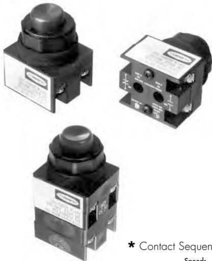
Hubbell's standard 22 mm pushbuttons feature polyester construction for superior corrosion resistance, and the #6 terminal screws have self-lifting captive wire clamps to accommodate #22 through 2 – #12 wires per terminal. The pushbuttons mount in a round 22 mm or 7/8" hole. These pushbuttons are rated for NEMA 1, 2, 3/3R, 4/4X, 12 and 13 installations and are UL/CSA approved.
